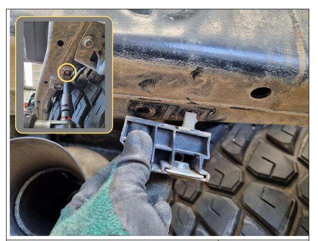
26. Remove and discard the 2x plastic lower bumper mounts on the underside of the chassis/towbar by removing 1x 12mm hex head bolt on each mount.
