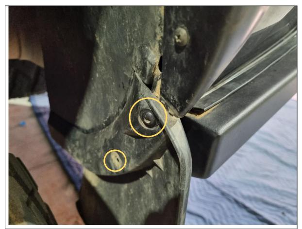
93. Refit the mudflap back to the bumper on both sides with the retained bolts and plastic push rivets.
