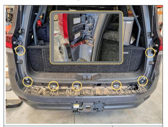
19. Using a 10mm socket/spanner, remove the 7x 10mm hex head bolts securing the top of the bumper to the rear of the vehicle.
