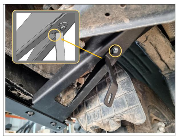
87. Loosely secure the side underpanel brace to the wing brace bracket with 1x M6x20 hex head bolt, flat washer and flange nut as shown.
