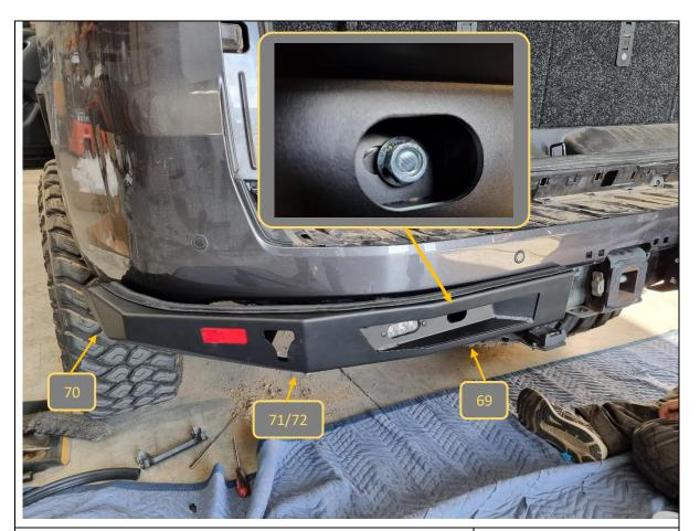
66. With assistance of another person, lift the wing up onto the vehicle. Ensure the M12 bolt fitted in the previous step fits through the slot shown.
