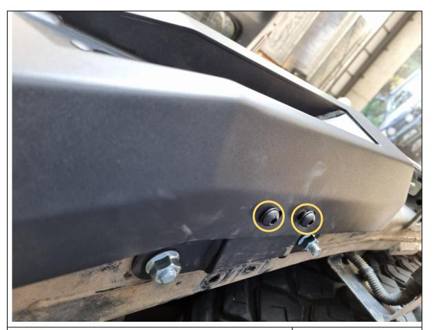
69. Loosely secure the bottom of the wing to the lower mount bracket with 2x M8x20 black button head bolts and washers.
