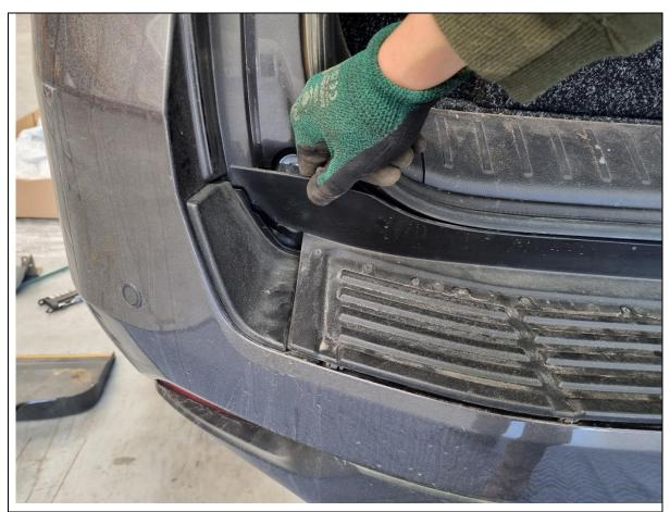
17. Starting from a top corner, pull upwards and outwards to remove the plastic tread panel. Set aside for later.
