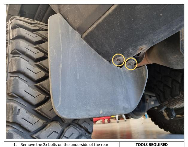
1. Remove the 2x bolts on the underside of the rear mudflap with a 4mm hex/Allen key.
