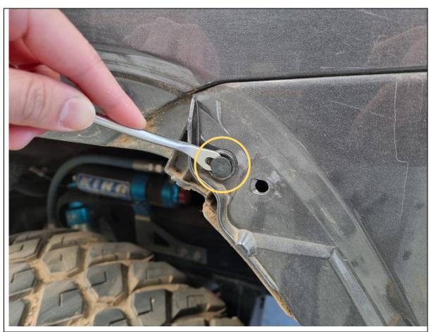
12. Remove the plastic push rivet securing the top corner of the rear bumper to the body on each side.
