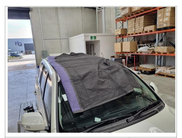
32. Place a soft blanket on the roof in between the roof channels to protect the paintwork while the roof rack is installed.
