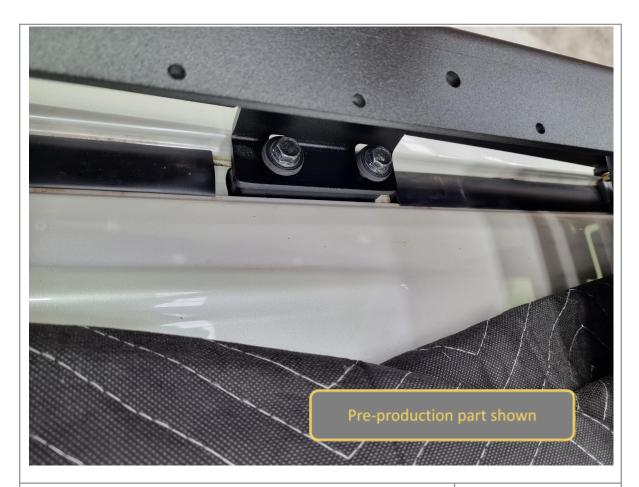
36. Loosely secure the roof rack to the roof with the long rubber sealed factory fasteners and supplied M8x50 hex bolts from the previous step.
