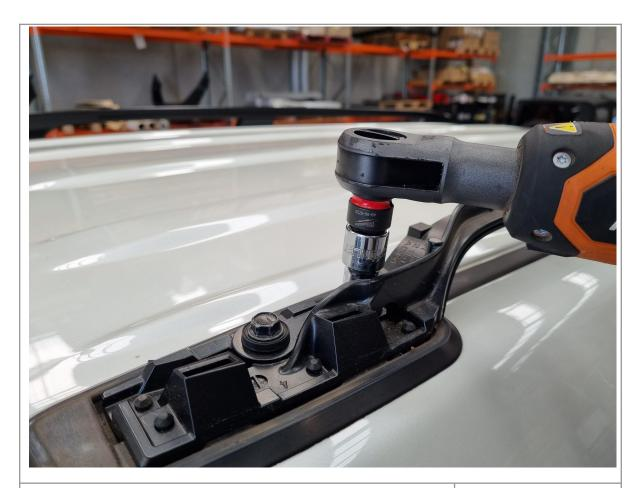
7. Remove the 4x 12mm head bolts securing the front and rear of the roof rail to the roof.
