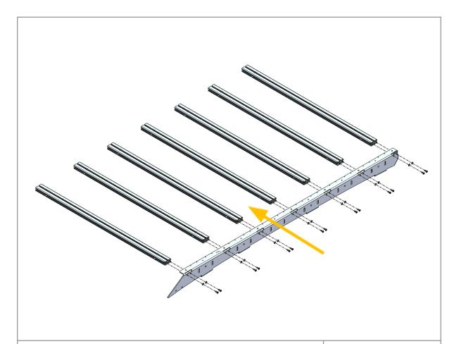
18. Fit the rack side plate to the extrusion.
