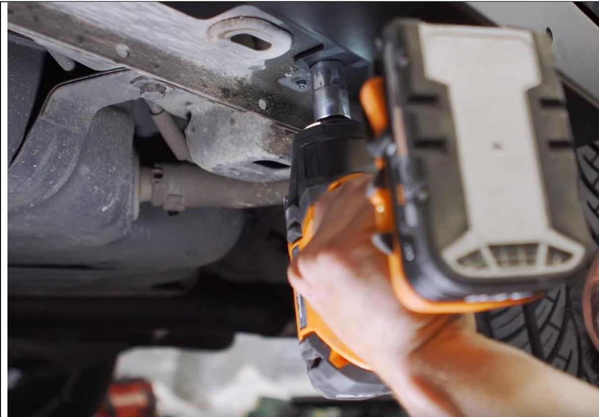
17. Once all bolts have been started, Torque down each bolt and screw
