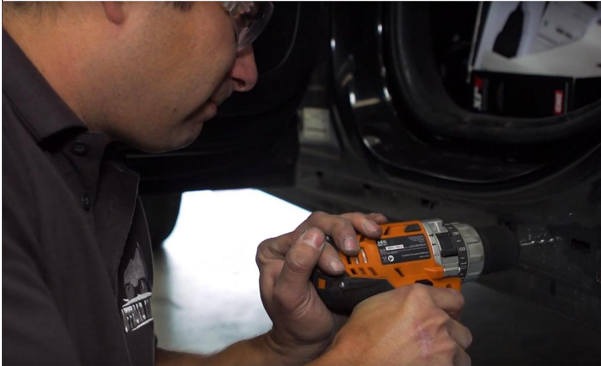
9. Drill out all marked holes. Holes on sides to 9mm (or imperial equivalent.) A 5mm pilot hole will make this step easier. On the side holes you will drill through two layers of steel.
