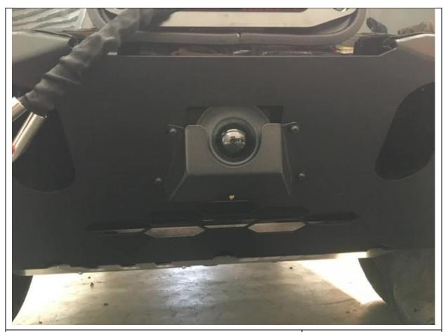
28. Secure ACC cover to main plate with M6 x 16 button head cap screws washers and flange nuts
