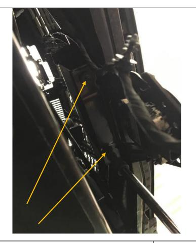
8. Remove Bracket that holes sensor
