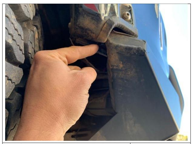
33. If your Jeep is equipped with parking sensors and they are going off as they see the new bumper you can fix this by adding a cable tie to the slot that originally holds the lower air damn being pointed to in the picture. Use the cable tie to pull this side of the bumper into the middle of the car. What this does is flex the bumper away from the new pre runner and points it in a slightly new direction.
