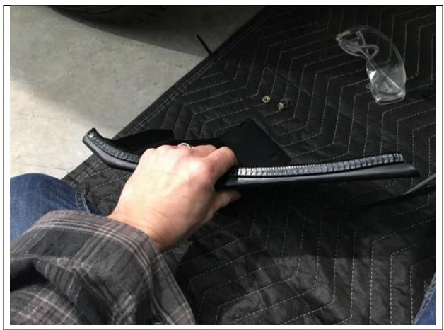
17. Fit pinch weld to top edge of wings like shown
