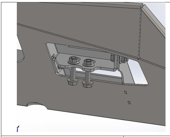
11. Fit Pre runner mounts as shown with M10 x 25 bolts, washers and flange nuts
