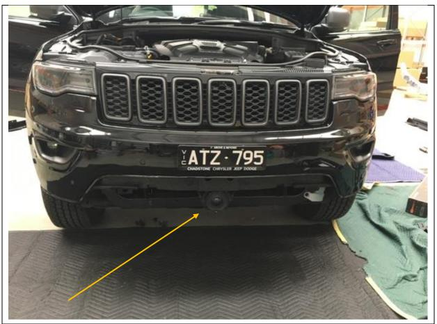
7. If Adaptive cruise control is fitted, unplug loom and pull sensor off posts
