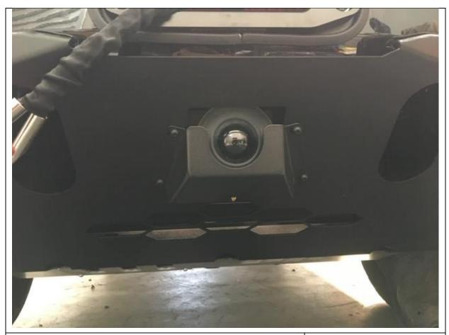
27. Secure ACC cover to main plate with M6 x 16 button head cap screws washers and flange nuts
