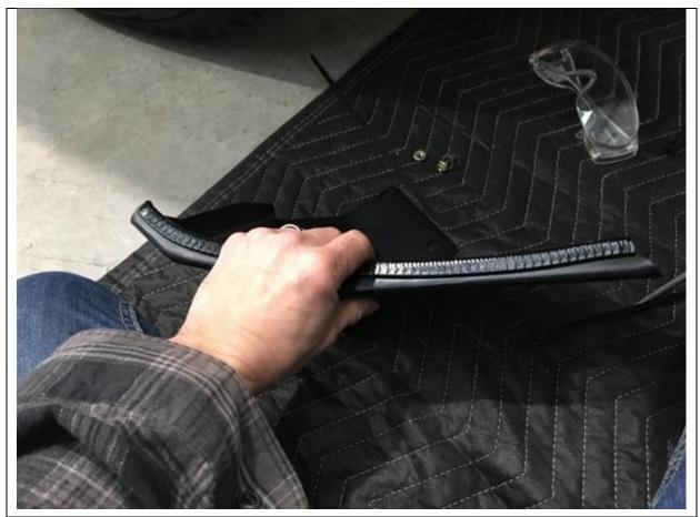
16. Fit pinch weld to top edge of wings like shown
