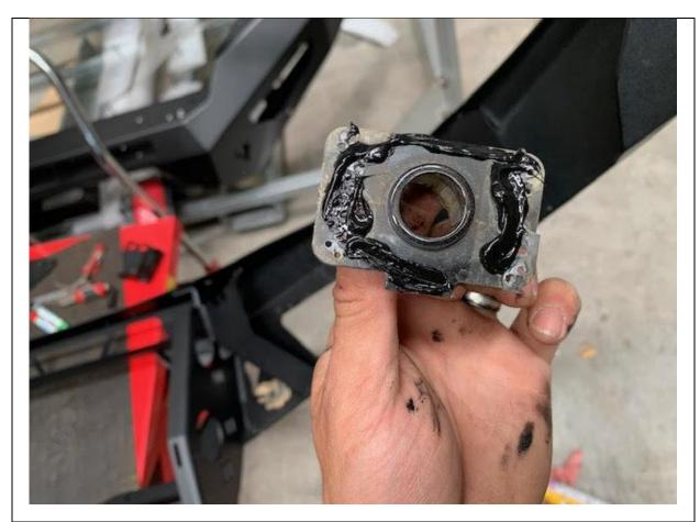
56. Clean the front face of the sensor mount and when dry apply a healthy amount of adhesive silicone to the front face of each sensor mount
