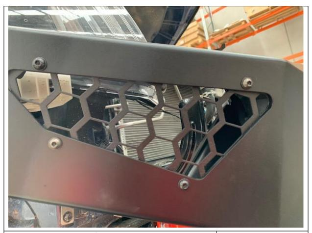
94. Fit mesh panel to bar from behind with M6 hardware
