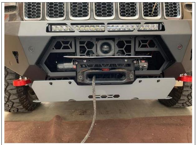
96. Fit bash plate as shown with M8 hardware through bash plate, mesh panel and into winch cradle.
