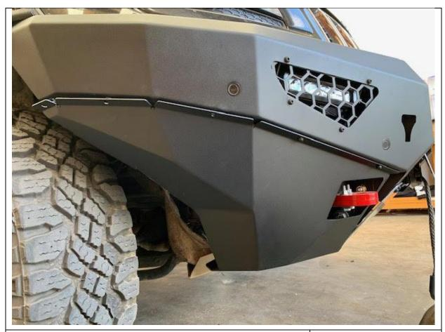
100. Fit under panels as shown with M6 along top edge and M8x 30 bolts. Trim Felt wheel well liner with razor blade so it tucks neatly behind the under panel which will hold it in place.
