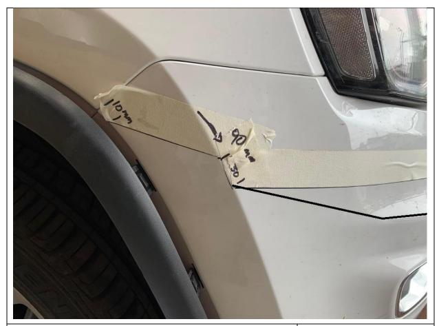
37. Use masking tape above the cut line to protect the bumper section you're going to keep
