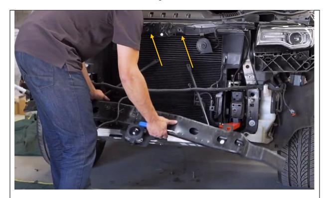
50. Remove 2x screws with 13mm tool holding round support bars from top of bonnet support then remove entire reinforcement bar.
