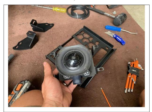
87. Fit ACC mount with Radar to centre mesh panel with M6 hardware
