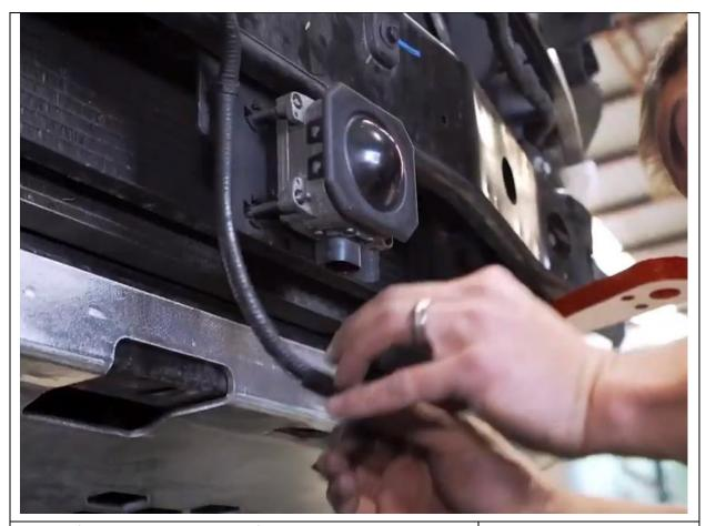
49. If Adaptive cruise control is fitted, unplug loom and pull sensor off posts
