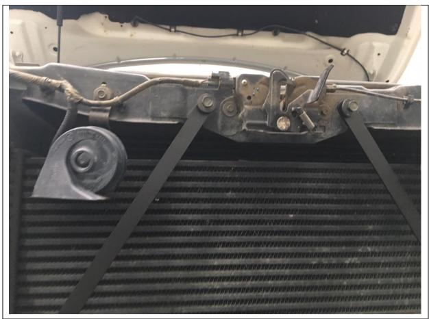
54. Fit radiator braces as shown with factory bolts
