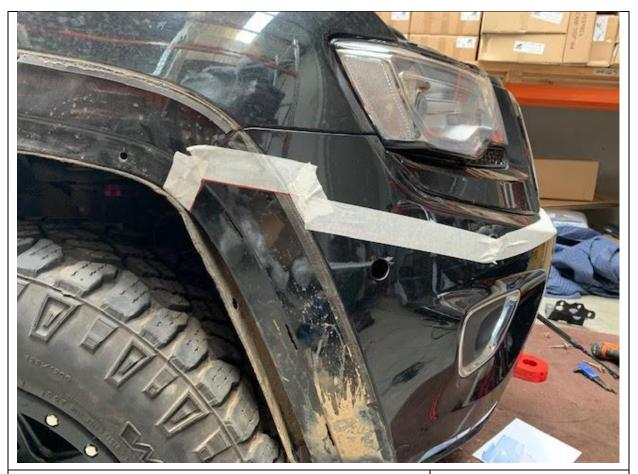
23. Use masking tape to mark out the cut lines. Put the masking tape above the cut lines to protect the portion of the bumper that will stay.
