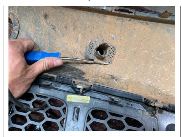
55. If factory parking sensors are present on the vehicle you'll need to remove the sensor from each housing and pry the housing off the bumper with a trim tool or flat head screw driver
