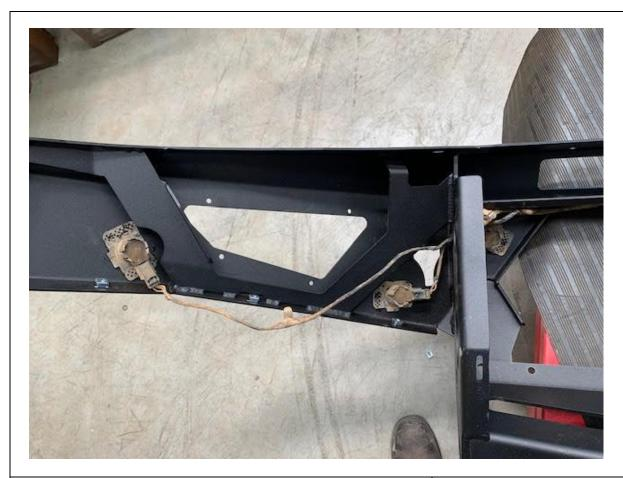
63. After at least an hour push the sensors into their housings. Make sure the housings are set, if the weather is cold you may need to wait longer.
