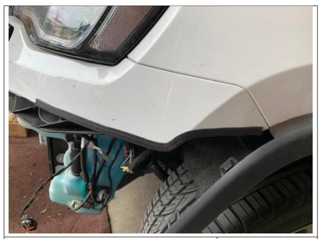
65. Fit a small section of pinch weld as shown
