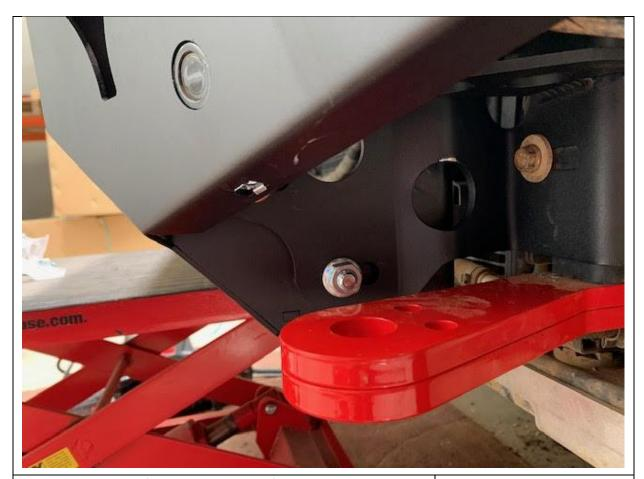
71. Fit the rest of the M12 x 30 bolts, flat washers and Nyloc nuts, leave loose for now.
