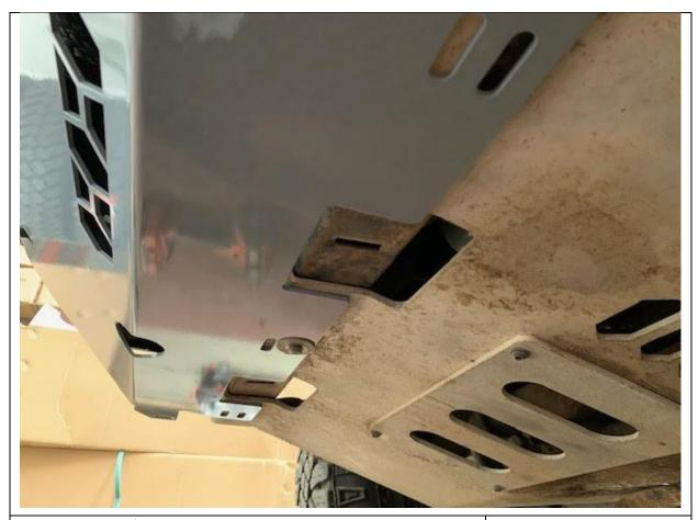
99. Fit lower factory M6 bolts through bash plate into cross member. Do not over-torque these
