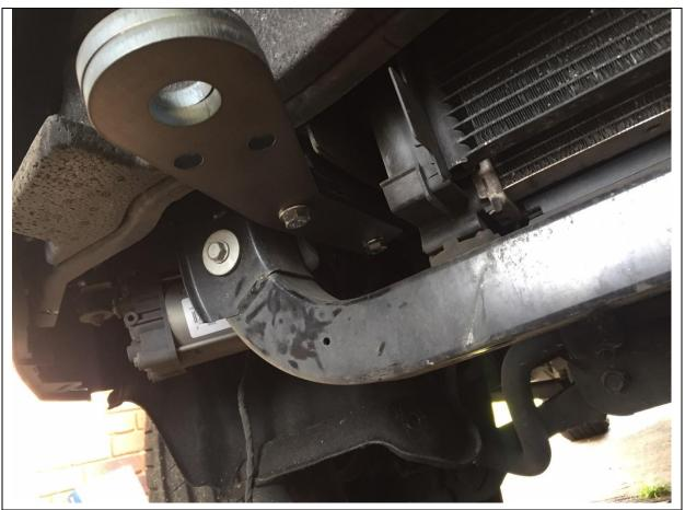
6. Fit Offroad Animal Tow points as shown on LH and RH side with M10x80 bolts directly into frame of Jeep. Torque down bolts to 70 Nm
