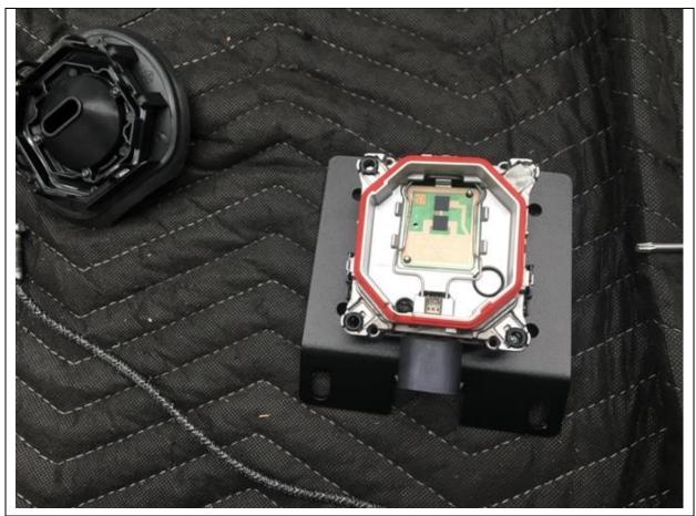
80. If My17+ model you'll need to remove the front face of the radar to get to the fasteners, and fit to ACC bracket
