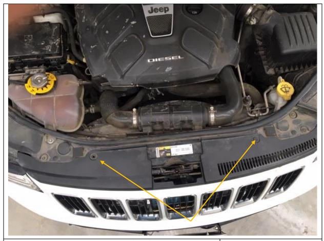
38. Next step is to remove the rest of the front bumper. Start with bonnet/hood open and pry out two clips shown with trim tool or flat head screw driver
