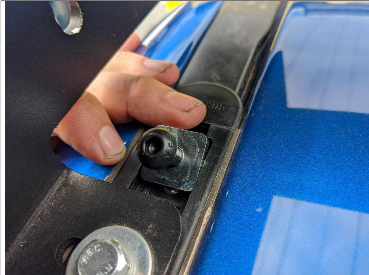
18. In preparation for fitment of the roof rack, Insert the Rhino Track nuts into the track fitted on the vehicle.
