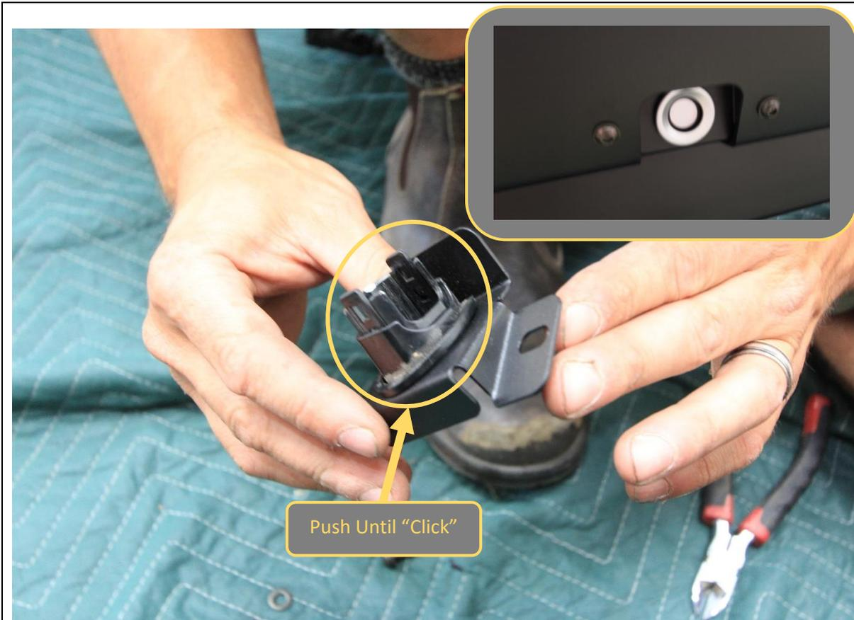
21. Fit the center housings into the sensor brackets. Insert outer housing from outside then replace inner bracket and press until an audible "Click" is heard.
