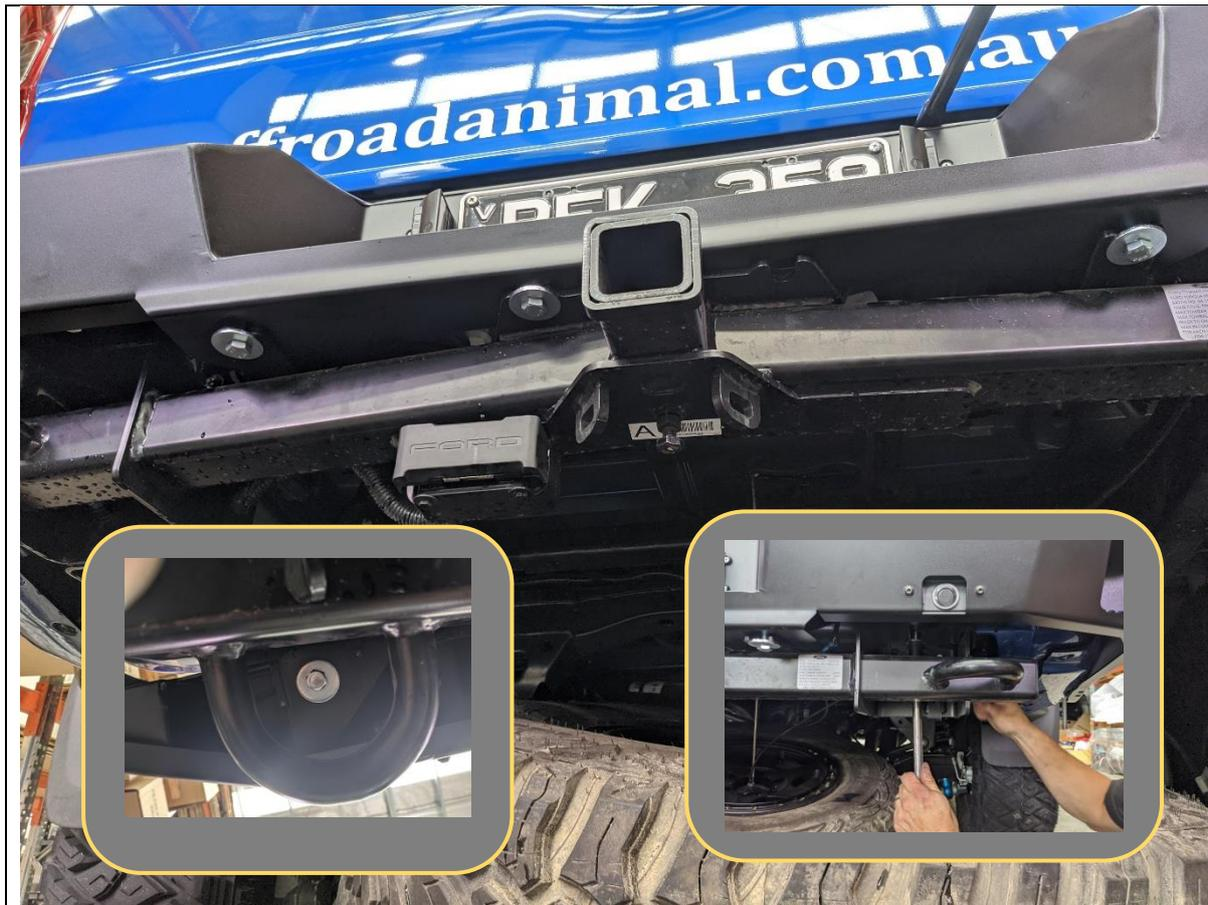
35. Secure Offroad Animal Bar to factory tow bar using M10x30 Bolts, M10 Large washers and M10 nuts in original factory locations.
