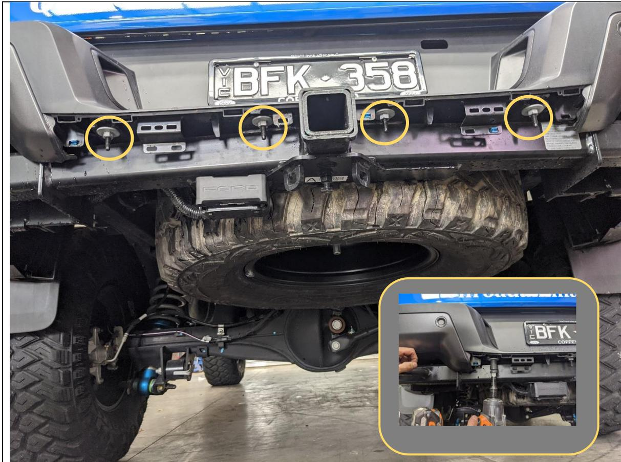
4. Remove 4x M8 nuts side securing the bottom edge of the rear bar. to the Chassis. Due to length of the studs use a deep socket for easy removal.
