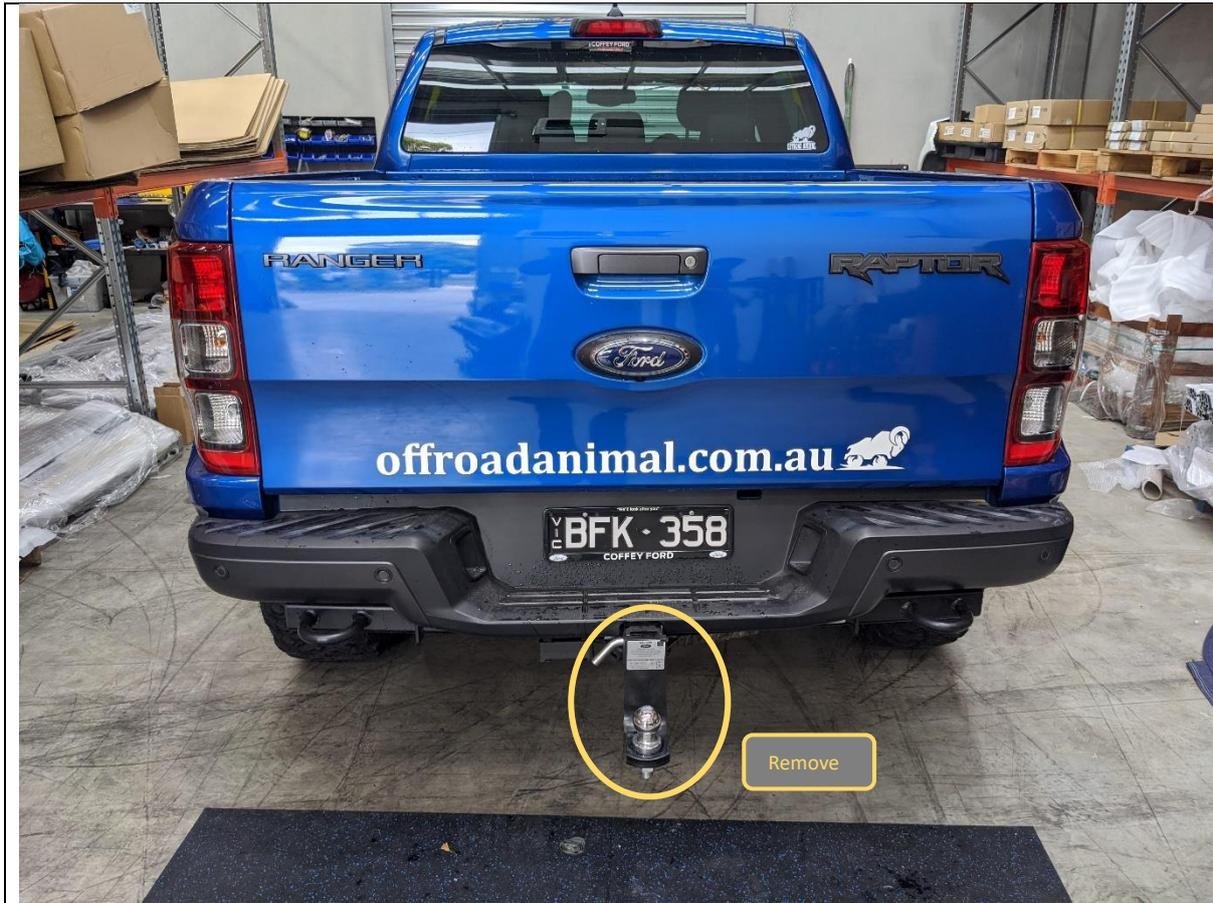
1. Before beginning work, remove factory TBM if fitted for easier access. 17mm spanner may be required to loosen anti rattle bolt on bottom of hitch.
