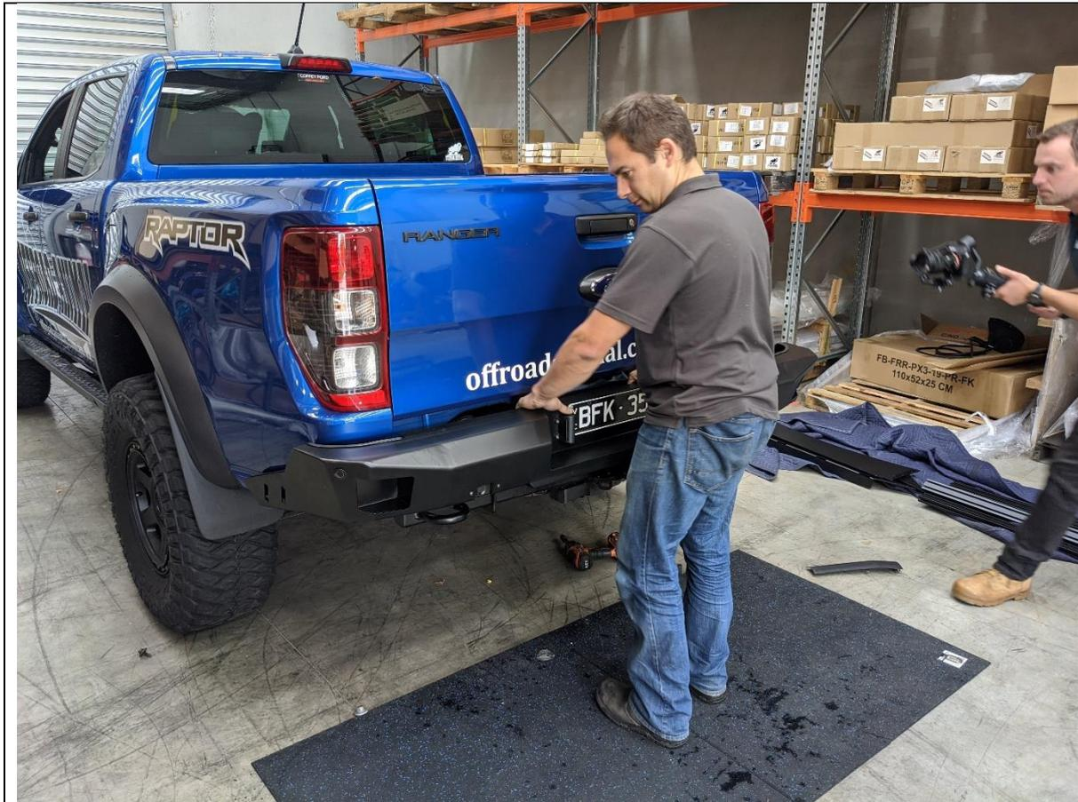
33. Lift the rear bar into position on the car. This can be done alone but will be easier with the assistance of another person. The bar should sit on top of the securing tabs on the tow bar.
