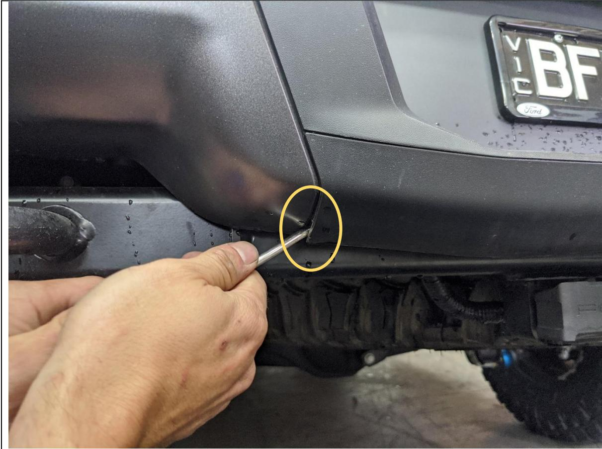
2. Remove the trim strip that conceal the bottom mounting bolts by levering corner with trim tool or flat head screwdriver as shown.
