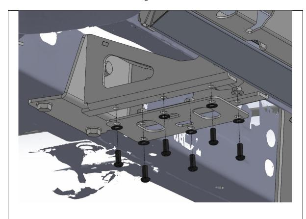
41. Once front mount bolts are tightened, fit the brace plate using 6x M8x20 Button Head, M8 Flat washers and M8 Flange Nuts
