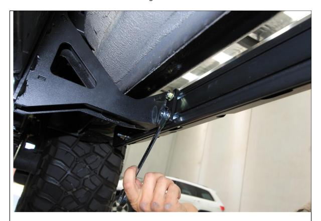
40. Tighten all mount to slider M10 flange nuts using 15mm spanner. A ratcheting spanner makes this process easier
