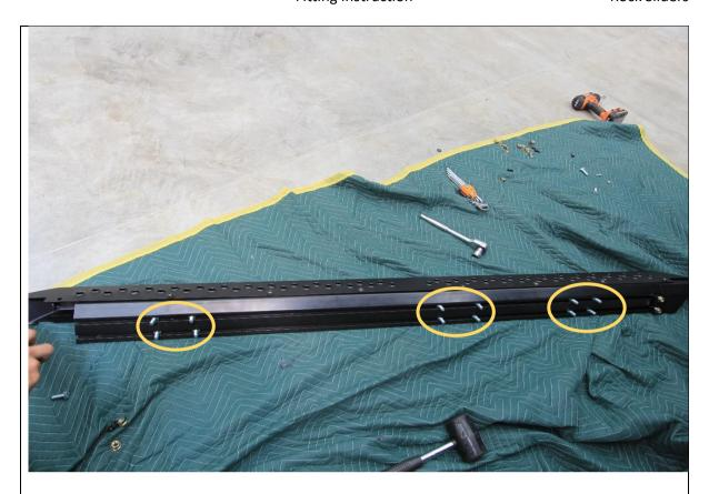
27. Slide the 12x M10x25 Hex bolts into the T slots on back side of extrusion. 6 bolts per slot.
