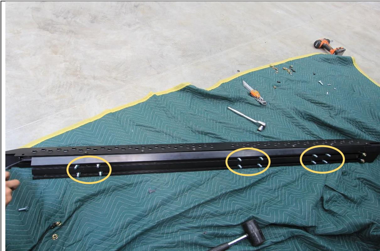
27. Slide the 12x M10x25 Hex bolts into the T slots on back side of extrusion. 6 bolts per slot.
