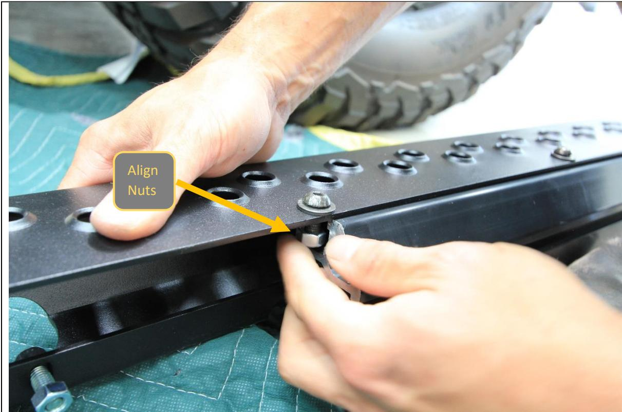
21. Slide the step plate onto the main slider structural extrusion. Align the nuts as they enter the T Slots on the extrusion.
