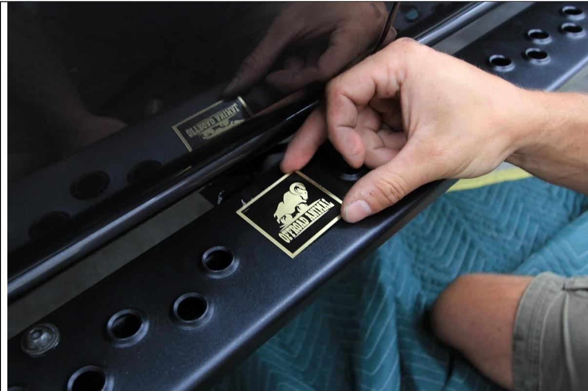
41. Fit the Offroad Animal logo plate to the small gap between pierced features on tread plate, using the pre applied double sided adhesive.
