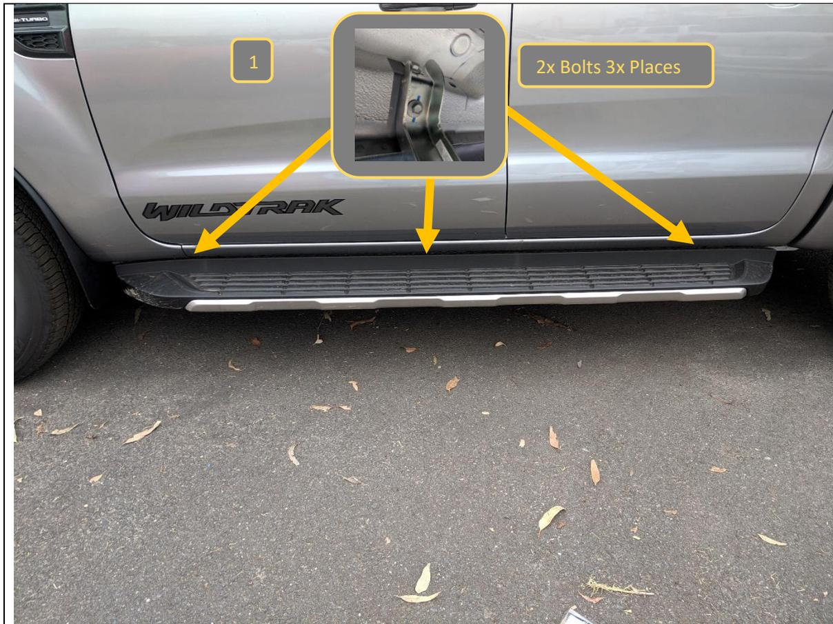
1. Remove Factory side steps if fitted by removing the 6x Bolts (2 Per mount) securing them to the body using a 12mm socket.
