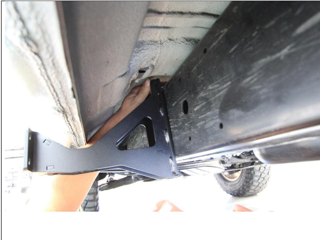
9. Prepare mid and rear mounts by pre-inserting the M12x125 Bolt, with flat washer, part way through the top mounting hole.
