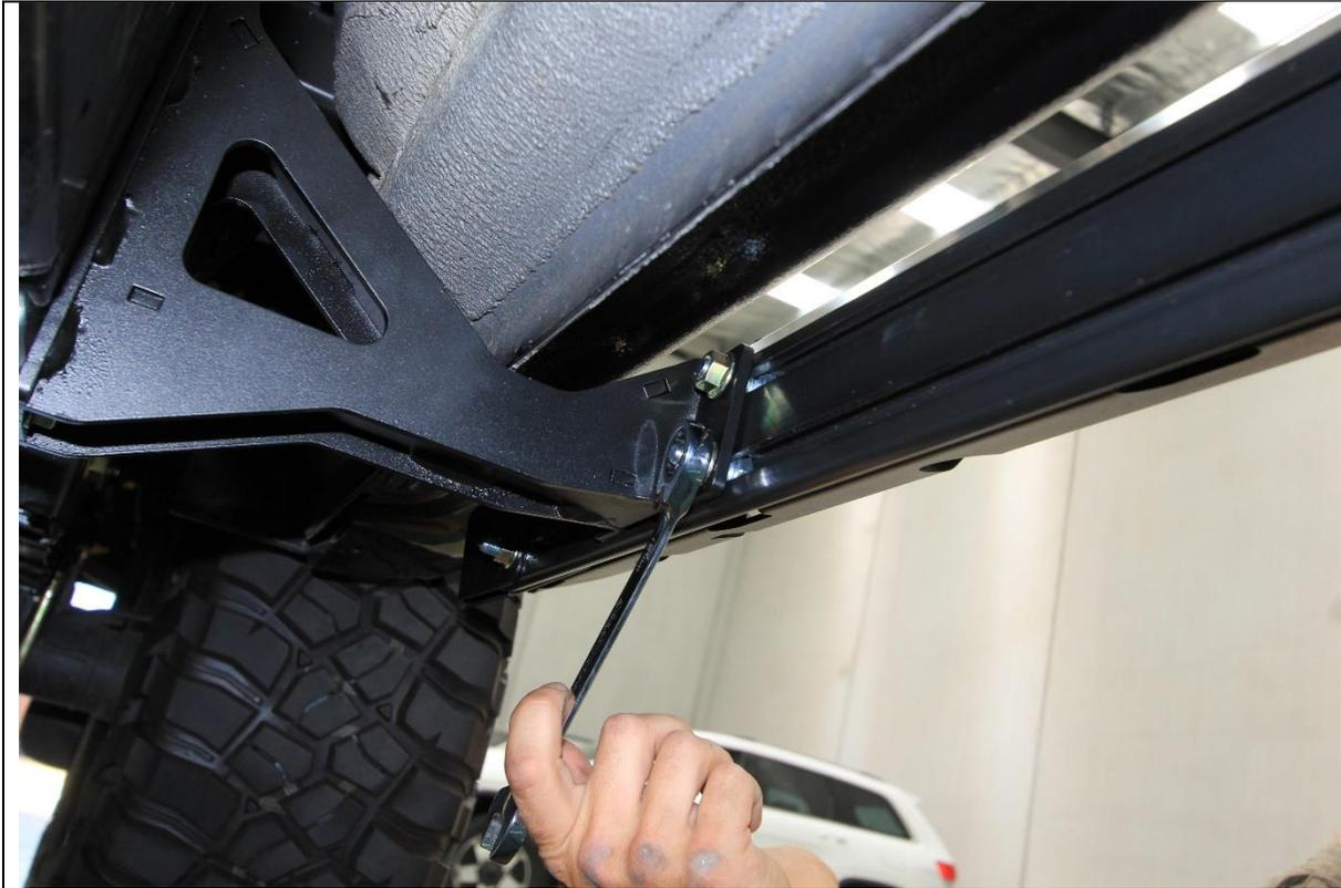
40. Tighten all mount to slider M10 flange nuts using 15mm spanner. A ratcheting spanner makes this process easier
