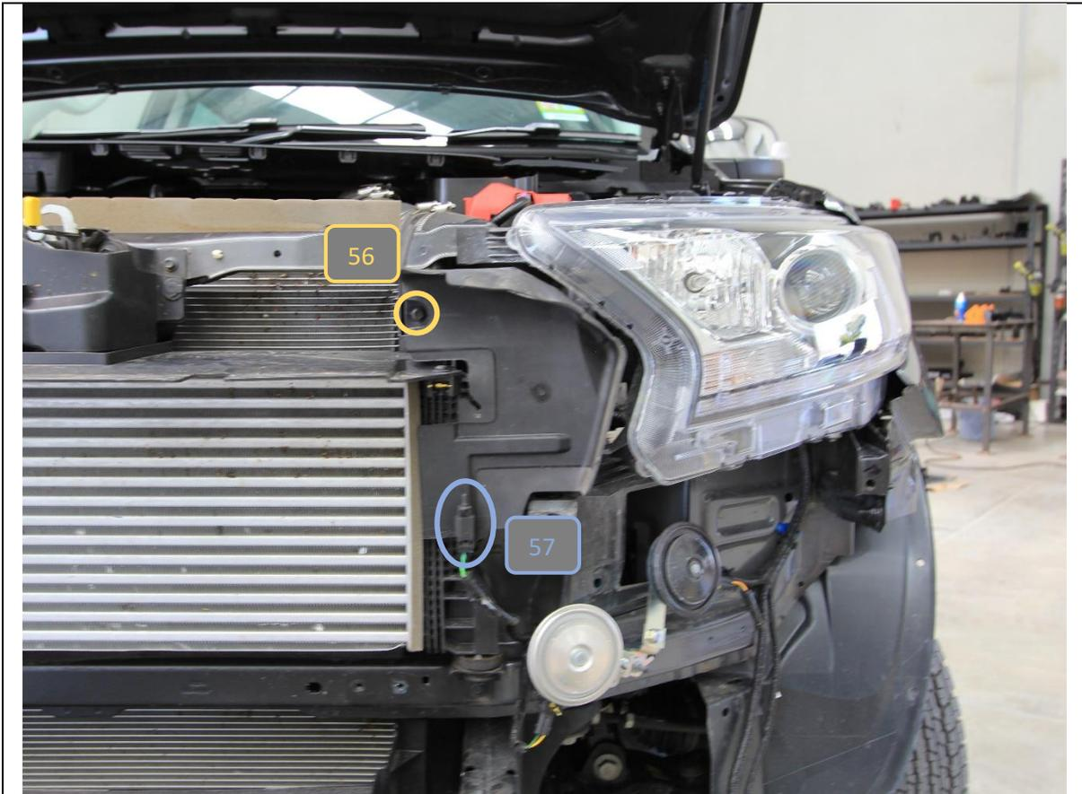
56. Re-Fit top portion of air guide using original bolt.
