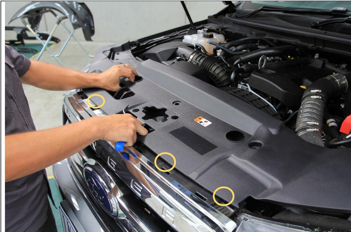
4. Carefully lift up plastic top shroud trim to unfasten concealed plastic clips securing trim to grille.
