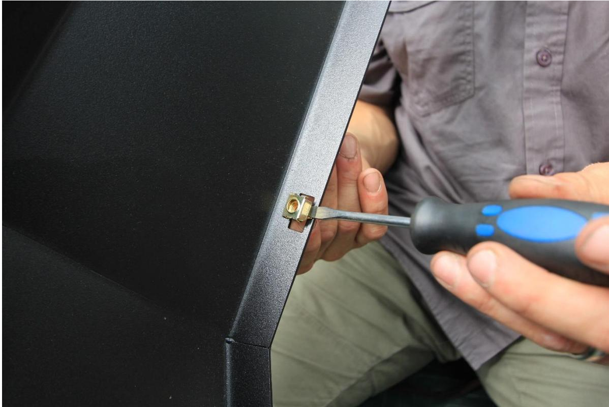
84. Insert cage nuts to square slots in bottom of wings. Seat cage nut against one edge of slot then push other edge in with flat bladed screwdriver.
