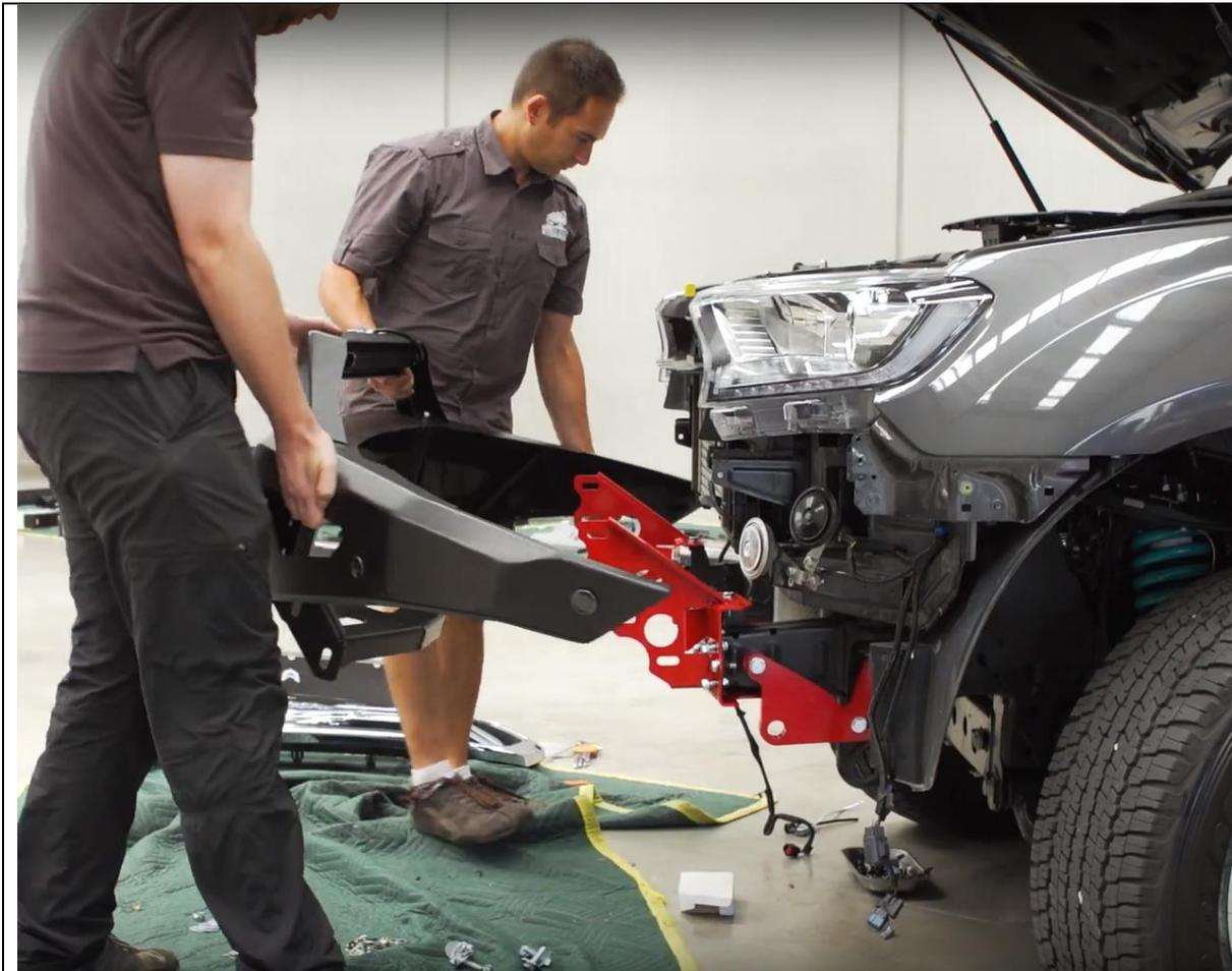
85. With assistance from either a lifting trolley or another person, Lift the bar up to the vehicle mounts.
