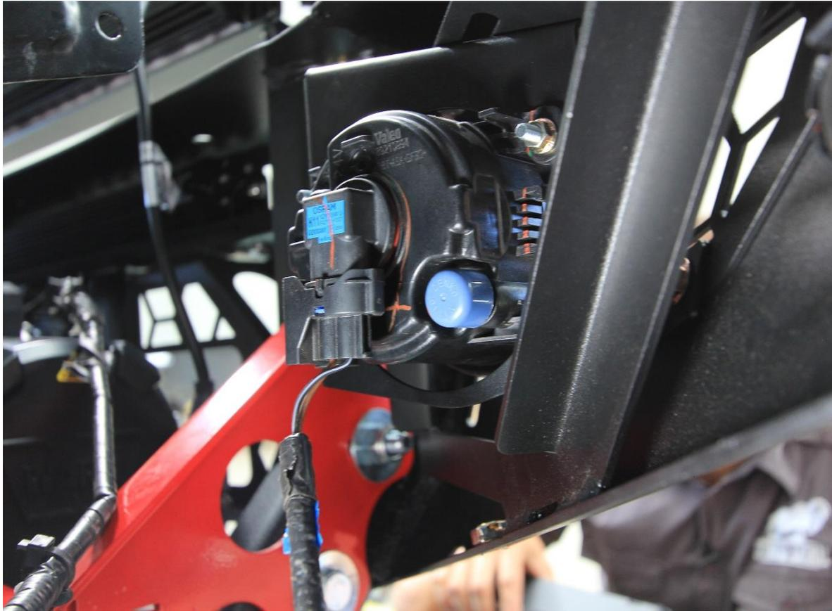
122. Reconnect fog light bulbs to housing, by inserting lamp at 90degree angle and rotating to lock in place. Repeat for both sides of vehicle.
