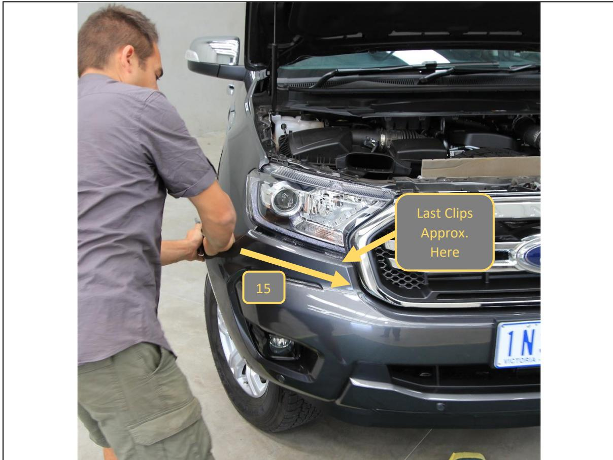
15. Starting at the wheel arch firmly but carefully pull the bumper away from the panel to release the clips.
