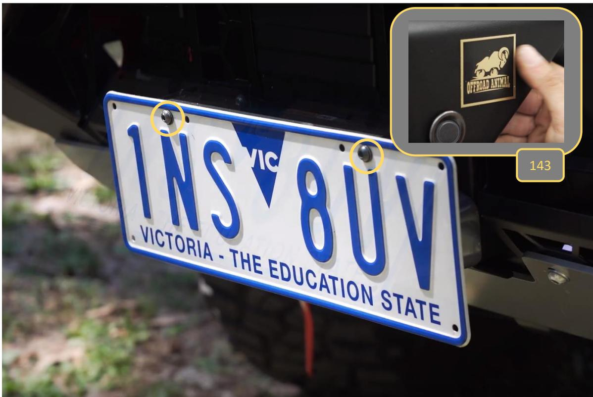
142. Re-Fit the number plate to the number plate flip, using the M5x15
