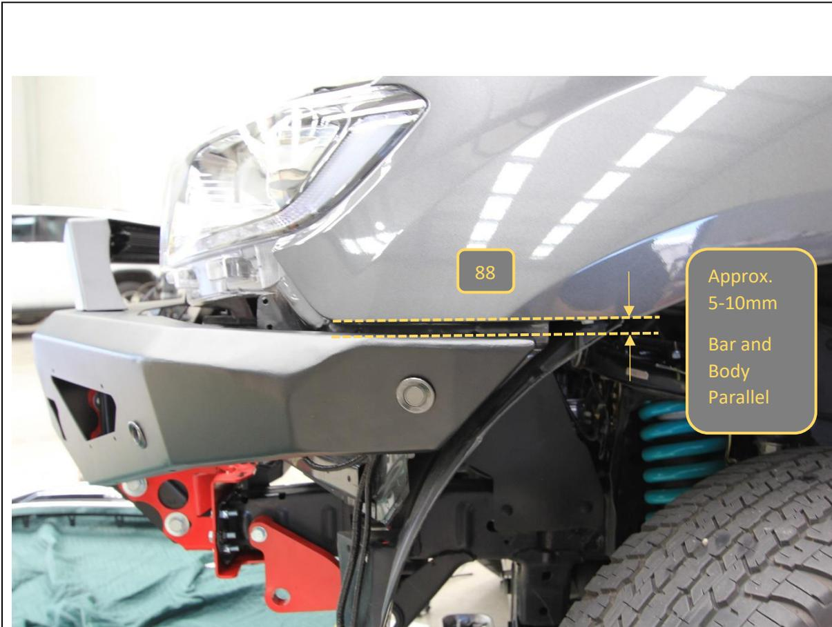
87. Fit the rest of the M12x30 bolts, Flat washers and Nyloc nuts to the bar to mount interface.
