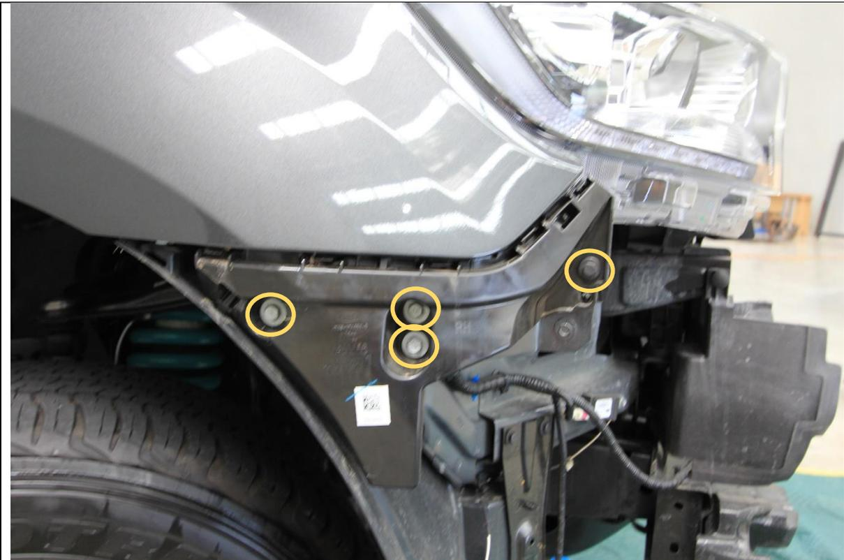
31. Remove the plastic bumper retainer by removing the 4 securing bolts using a 10mm Socket.
