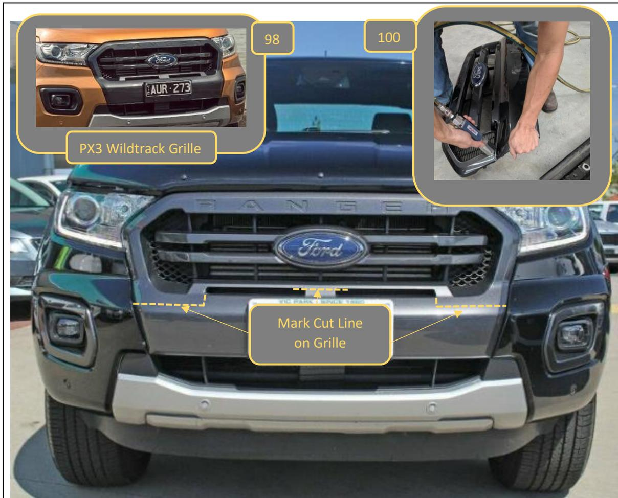
99. Wildtrack grille is different to XLT and lower models and needs to be trimmed to fit with new Offroad animal bar.
