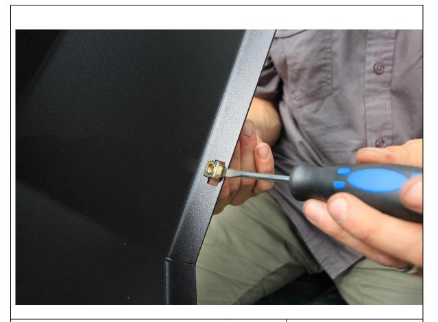
86. Insert cage nuts to square slots in bottom of wings. Seat cage nut against one edge of slot then push other edge in with flat bladed screwdriver.
