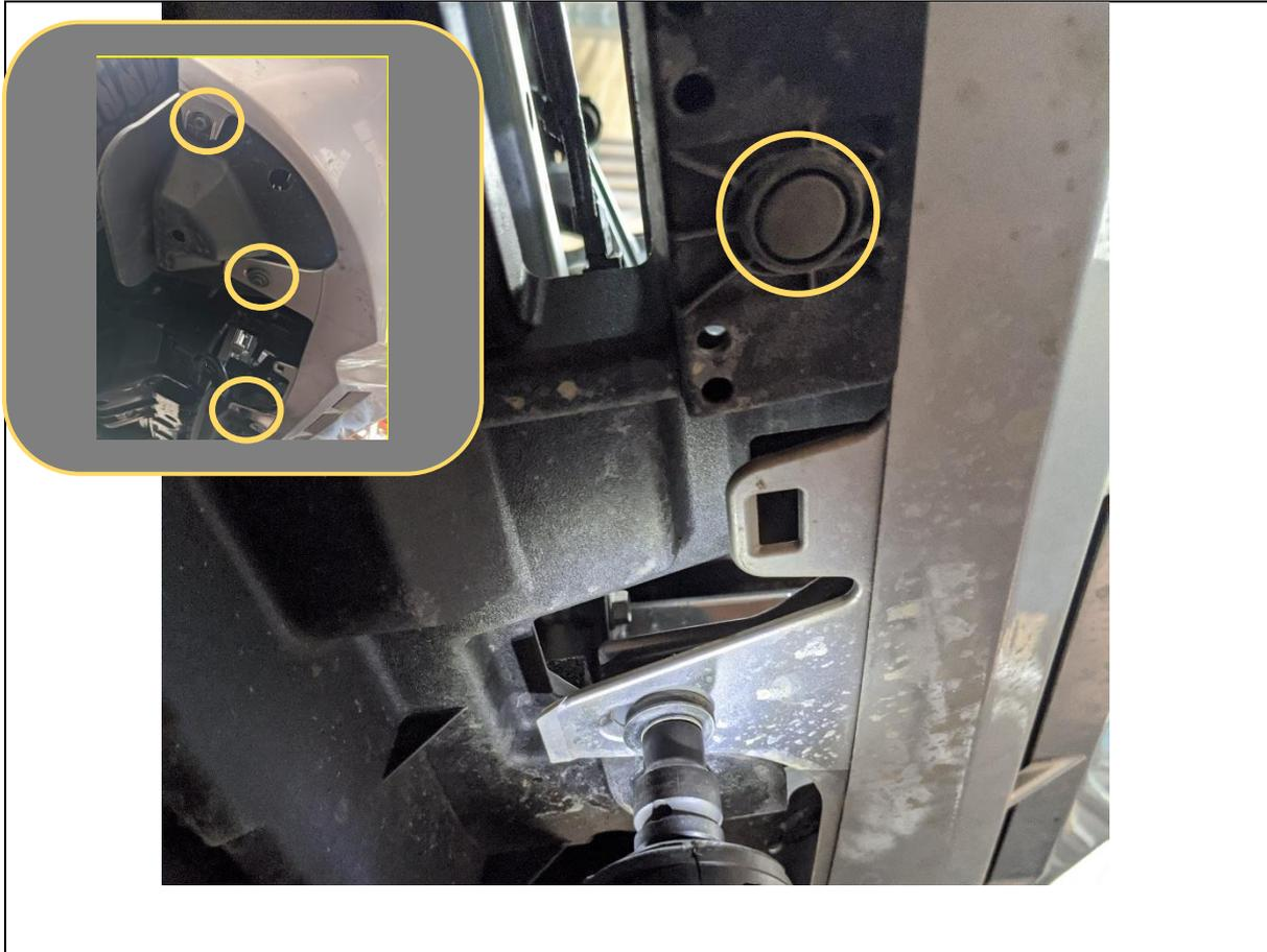
12. Remove the 10mm head screws securing the bumper to the underbody bash plate.
