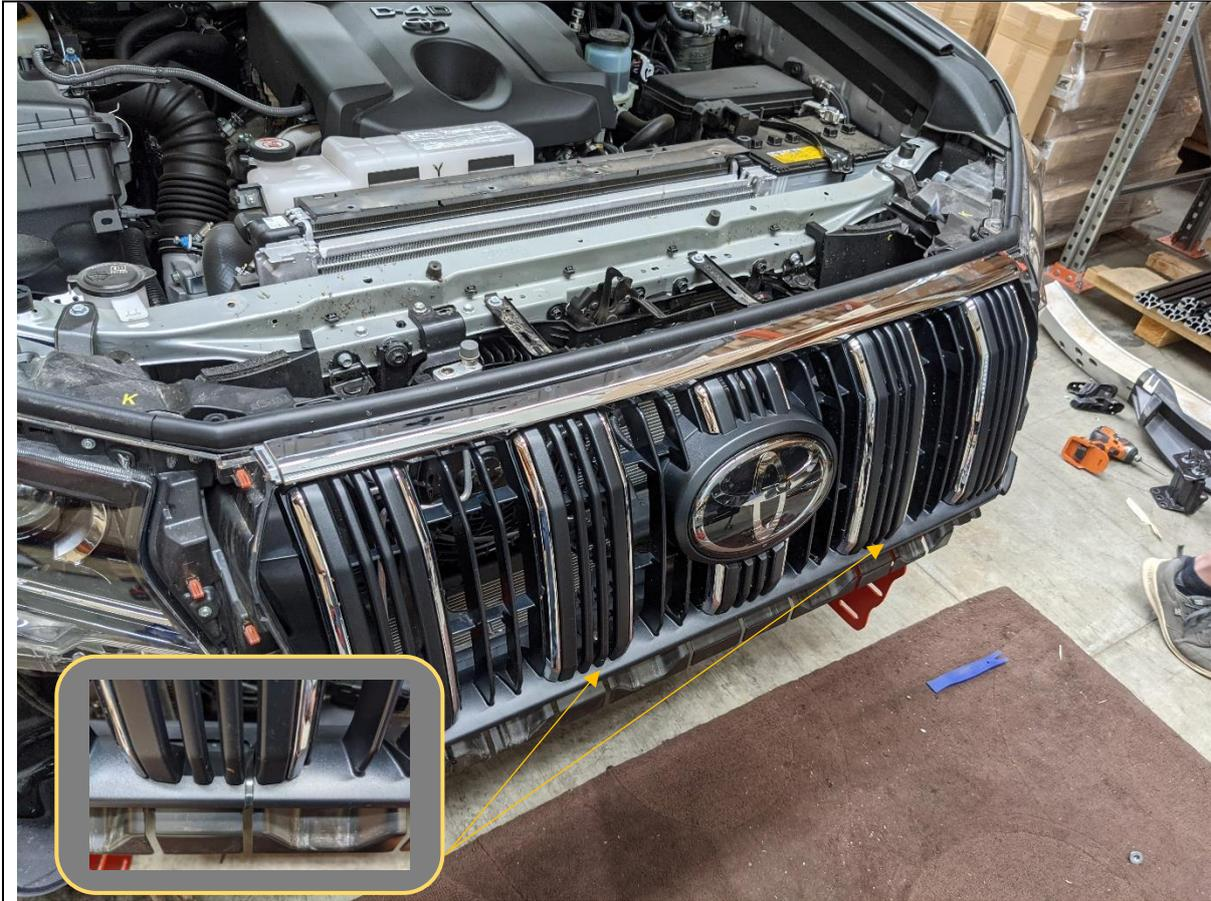
20. Re-Fit grille to vehicle, Secure the top of grille using the factory fasteners removed earlier.
