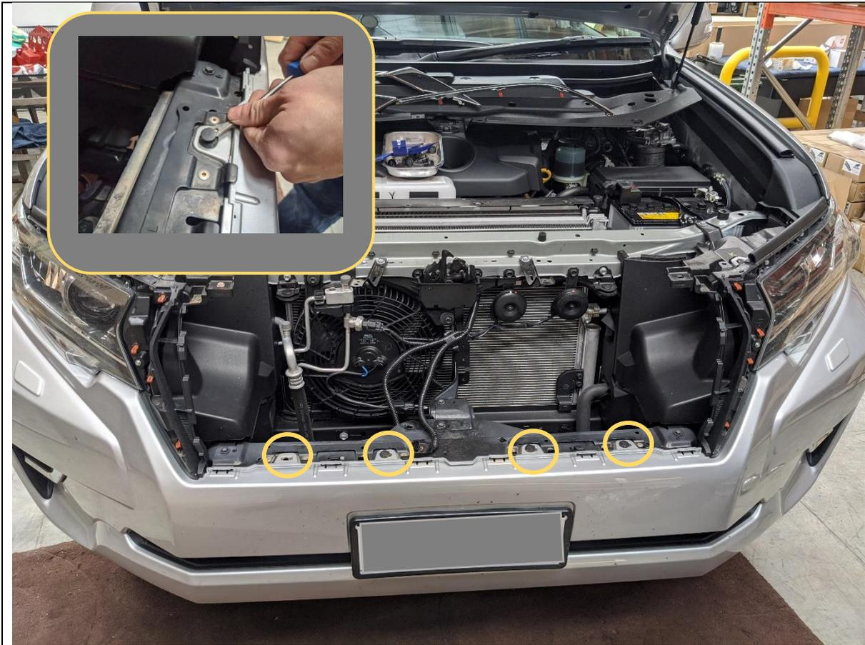
11. Remove the 4x Clips securing the bumper to the body crossmember
