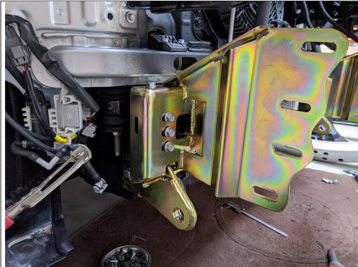
49. Loosely fit the Impact mounts to the chassis, re using the original factory flange Bolts.
