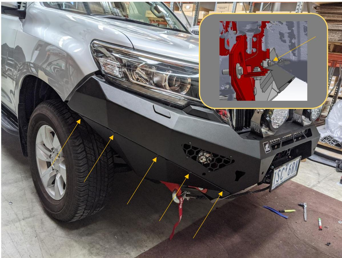
106. Fit Side Under panels (U-0029L/R) using, M6x16 button head and flat washer into the cage nuts placed earlier.
