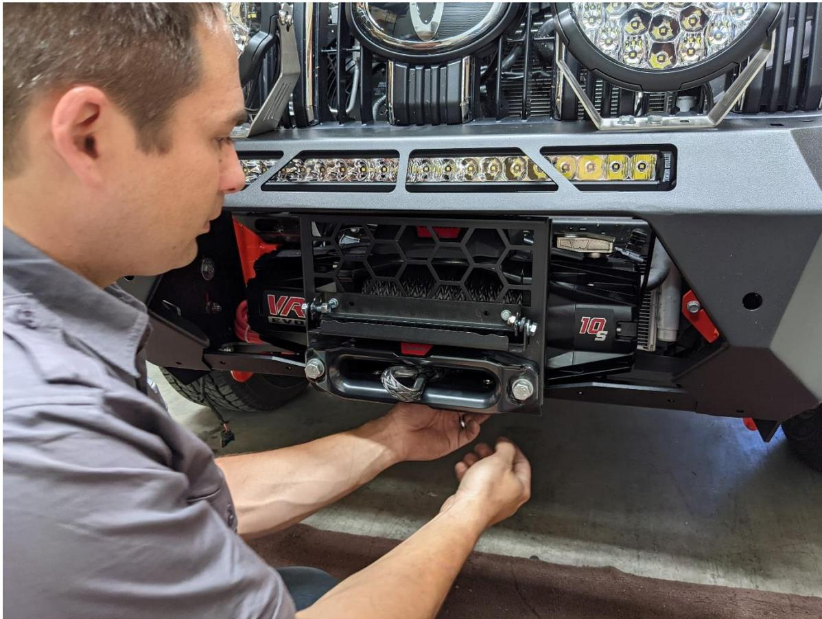
89. If Required, Fit winch fairlead to Mesh Fairlead Mount (M-0014). Use M10 or 3/8" Fasteners supplied with winch. The bar is only compatible with Hawse type fairleads.
