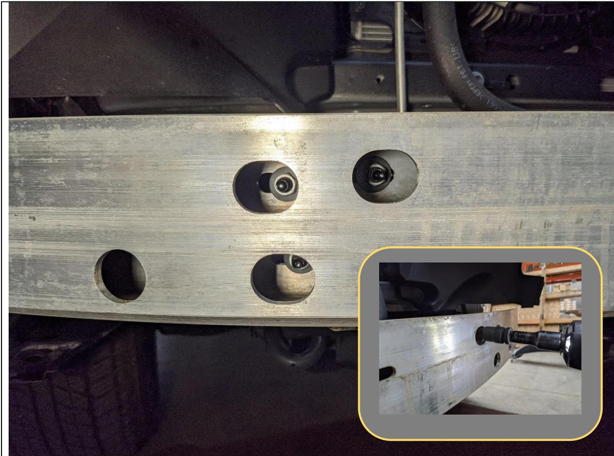
39. Remove the 6x 14mm head Nuts holding the impact beam to the impact beam brackets.
