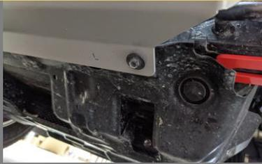
Production Spec – Factory Bolt and M8x30 Button Head
