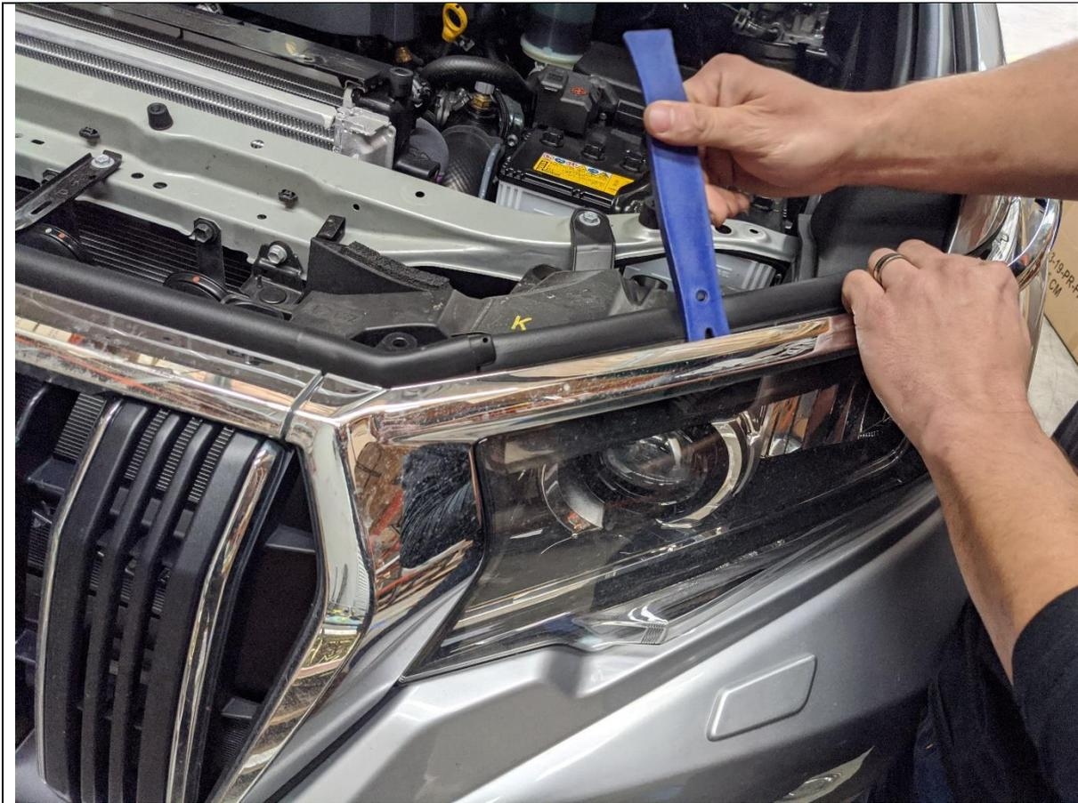
6. Using a rag or plastic tool to protect the chrome finish, carefully pry the L shape headlight trim to release the clips.
