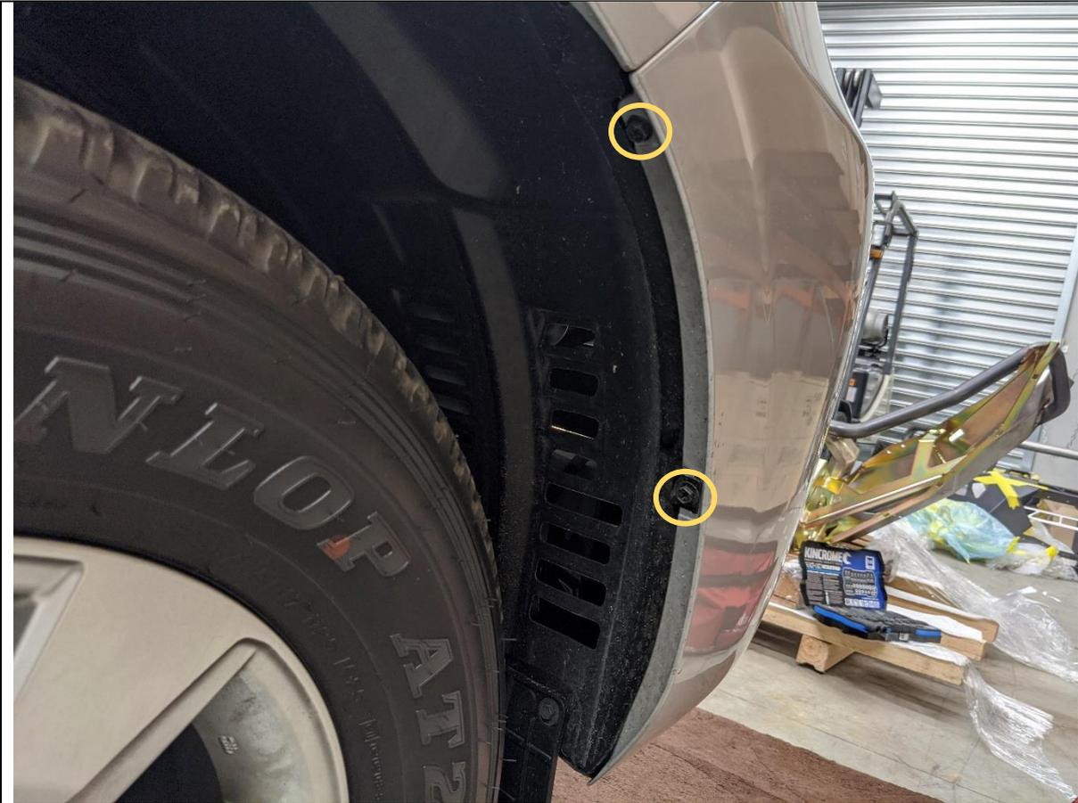
14. Remove the 10mm / Phillips screws securing bumper to the wheel arch liner.
