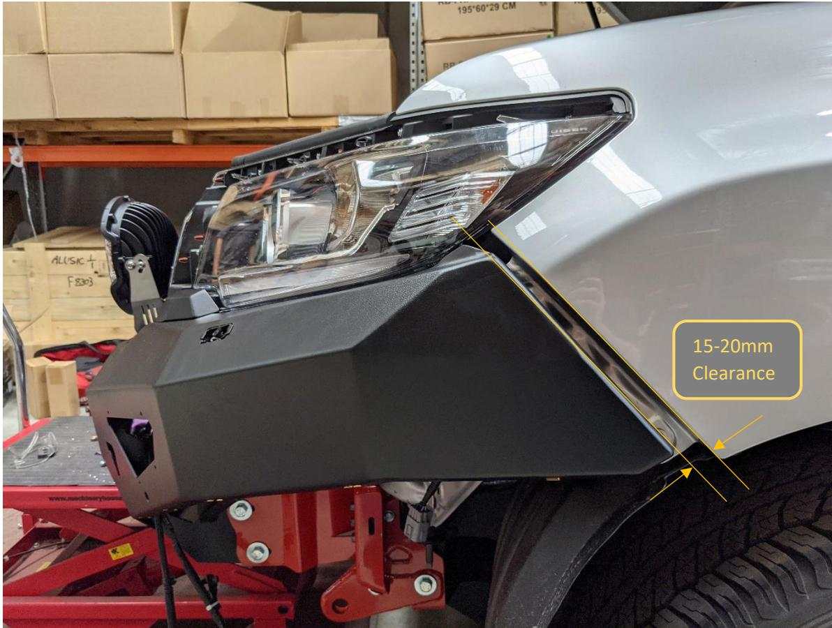
80. With assistance, from another person, Align the bar with the edges of the vehicle. Adjust such that the clearances are neat and even side to side.
