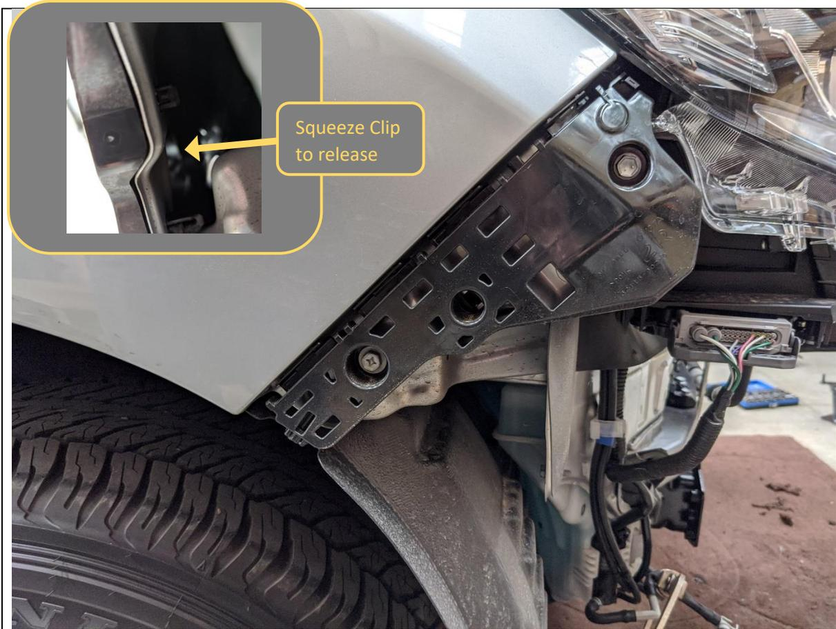
41. Remove the plastic bumper retainers by removing the Philips head and 10mm head screw, then prying out the large clip from behind using trim tool
