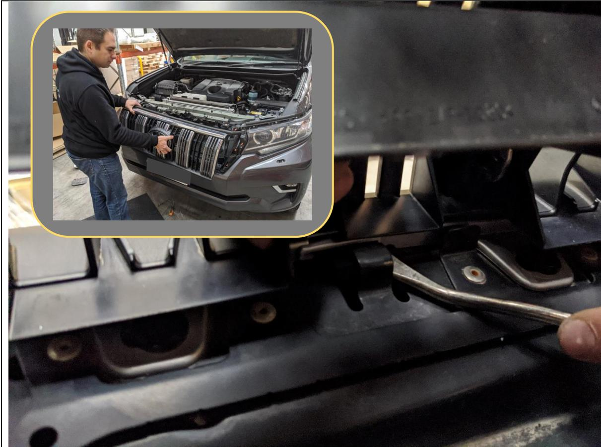
9. Using a trim tool pry open the clips securing the bottom of the grille to the bumper.
