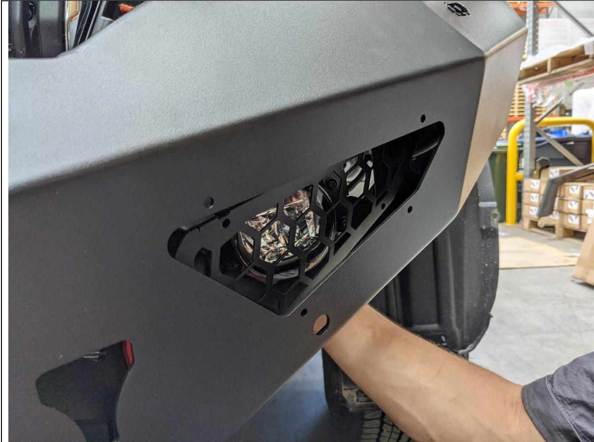
97. Fit Light cover mesh to bar using 4x M6x16 Button head bolts, Flat washers and M6 Flange Nuts
