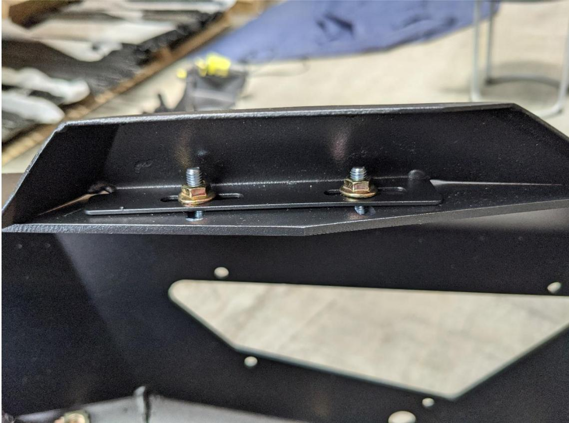
66. Pre fit the headlight infill panels to the top face of the bar, using M5 Button head screws, M5 Flat washers, and M5 Flange nuts. Secure finger tight at this stage
