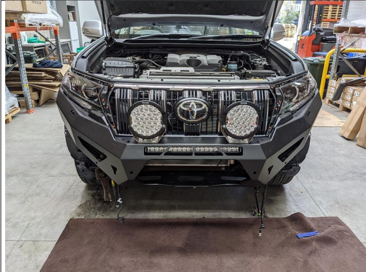
78. With assistance, either from another person, or a lifting trolley, lift the bar onto the mounts on the vehicle.
