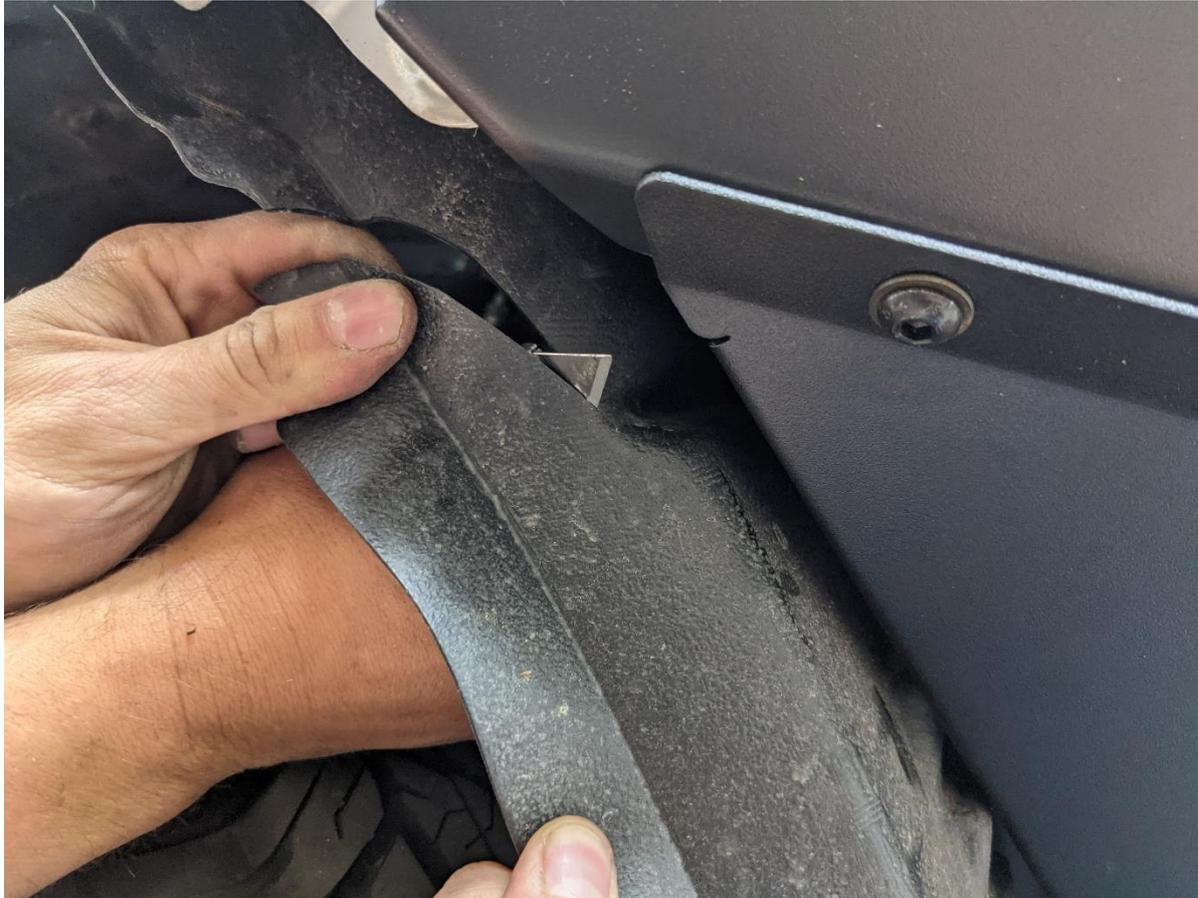
110. Using the edge of the under panel as a guide mark the wheel arch liner, approximately 15mm beyond the intersection of the under panel.
