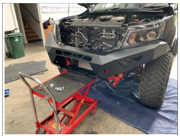
28. With the aid of a lifting table or a friend, lift bar onto vehicle
