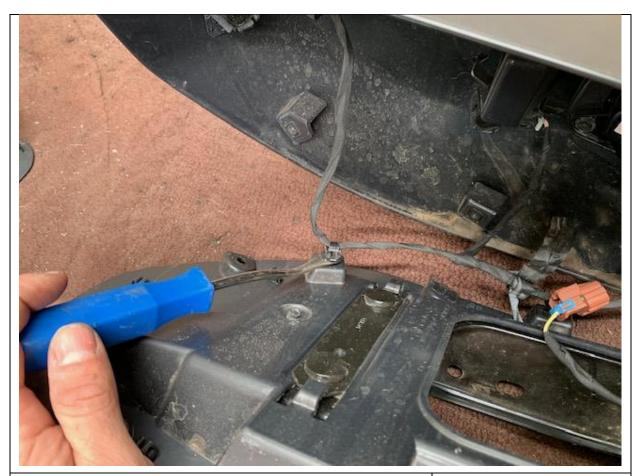
11. Remove all retaining clips for wiring
