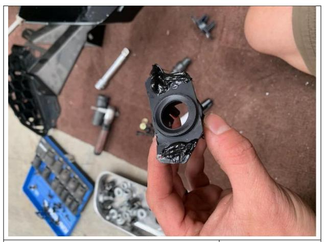
13. To refit the sensor to the bull bar, you'll need to dab the front of the housing like shown with adhesive silicone. However, you'll need to do a dry fit in bumper before this step to ensure you know sensor orientation.
