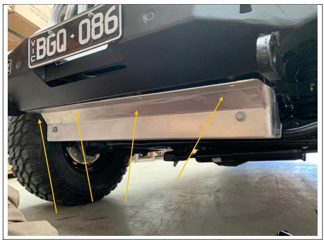
30. If fitting optional skid plate, hold plate up to bottom of bull bar and start the 4 x M8 x 30 button head cap screws with washers to hold plate in place, and re use hardware for the front
