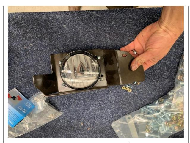
17. Fit Factory fog lights to Fog light brackets as shown using supplied M4 hardware
