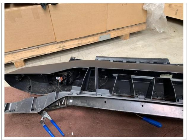
10. Once all screws haver been removed, you'll need to separate the inner bumper from the outer shell.
