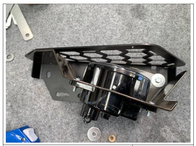
19. Fit fog light bracket to mesh panel like shown using M8 hardware
