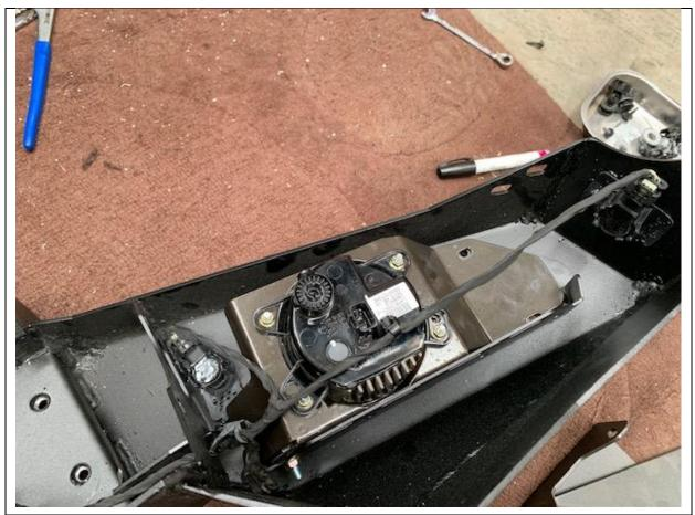
20. Fit mesh panel and fog light to bar and secure with M6 black button head cap screws washers and flange nuts
