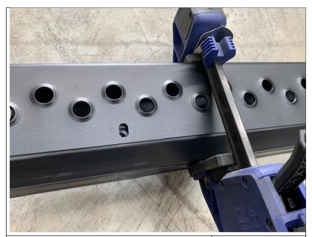
29. Using long tool feed nuts in to centre first and thread in with black M8 button head cap screws and washers
