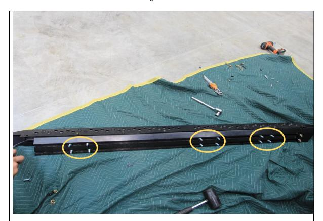
34. Slide the 12x M10x25 Hex bolts into the T slots on back side of extrusion. 6 bolts per slot.
