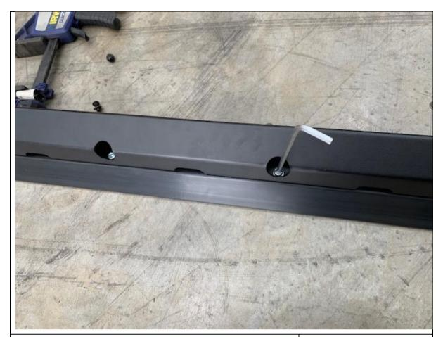
26. Thread cap screws into each hole
