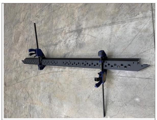
27. Flip entire slider up as shown28. Clamp step hard to extrusion
